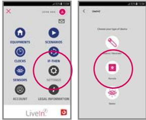
**1-** In the LiveIn2 app, from the SETTINGS menu, add a device BHz «Remote». Let you guide by the application to pair the transmitter with its PROG button.
