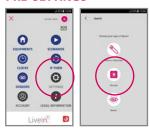
1 - In the Liveln2 app, from the SETTINGS menu, add a device BHz «Remote». Let you guide by the application to pair the transmitter with its PROG button.
