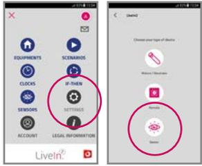
**1-** In the LiveIn2 app, from the SETTINGS menu, add a device BHZ «Sensor». Let you guide by the application to pair the sensor with its PROG button.
